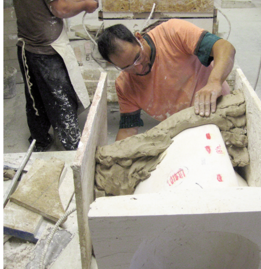
Fig. 1. Hand-packing clay into a plaster mold at Gladding McBean factory in Lincoln, California, 2014. All photographs by Edward Gerns..
