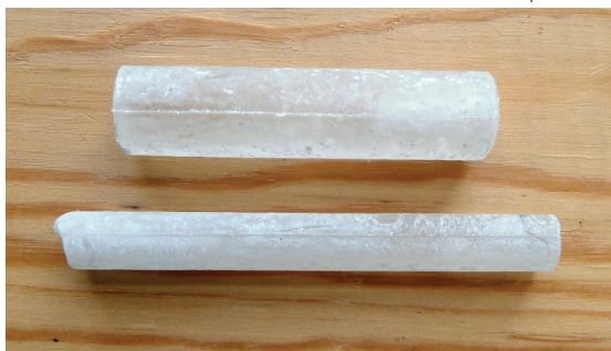
Fig. 7. Borate rods are available in a range of sizes including the 0.75 inch (19 mm) and 0.5 inch (13 mm) diameters shown here. Courtesy of Stan T. Lebow and the U.S. Forest Products Laboratory.
