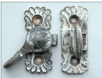
Fig. 4. Oliver Judd, "Patent Burglar Proof Sash Fastener," ca. 1865. The hinged hasp (at right) is brought down over the vertical turn button. The lever is then turned by means of an eccentric shank that draws the two sash firmly together. Photograph by author.
