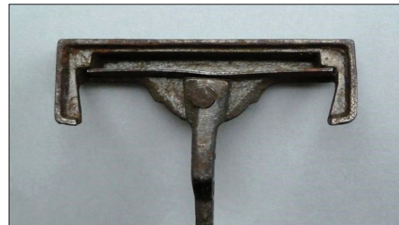
Fig. 2. Morton Judd, sash fastener, ca. 1847. The improvement was to add a flat spring that engages the flat end of the lever to hold it in place. Unlike the British quadrant-style sash fastener, the lever could be swung 90 degrees in either direction to disengage the keeper. Photograph by author.
