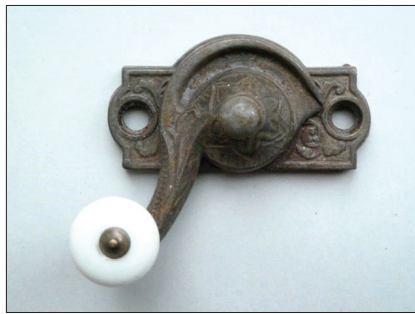
Fig. 5. Otto F. Fogelstrand, sash fastener, ca. 1877. This device incorporates a lever with a large hub at one end into which is cast a recessed eccentric groove. As the lever is turned, the groove engages a post or lug in the keeper (removed to reveal the groove) and draws the sash together. Photograph by author.
